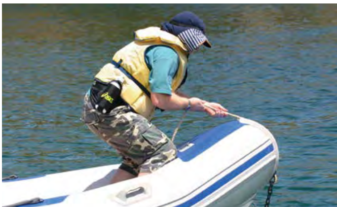
Use the buoyancy of the hull to assist when retrieving a snagged anchor
