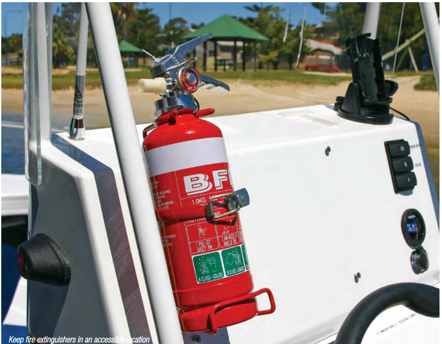
Check the gauge is in the green
